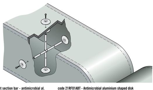
code 21RF02ABT - Reinforcement section bar - antimicrobial al.
