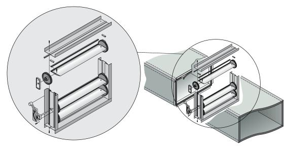
code 21SR01 - Double vane section bar for modular damper
